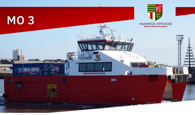
Designed by Walker Marine Design, UK — The MO3 was designed and built to perform a multitude of tasks, including crew transfer, offshore bunkering and cargo operations. Capable of transferring personnel in 1.75 Hs, the MO3 is one of only a handful of vessels that are capable of achieving this milestone in passenger transfer.
