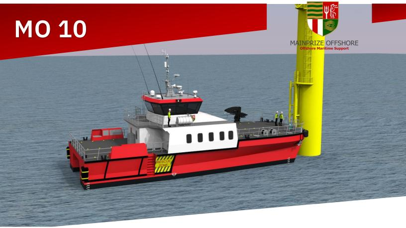
Designed by Walker Marine Design, UK – The MO10 was designed and built to perform a multitude of tasks, including crew transfer, offshore bunkering and cargo operations. Capable of transferring personal in 2m Hs, the MO10 is one of only a handful of vessels capable of achieving this milestone in passenger transfer.
