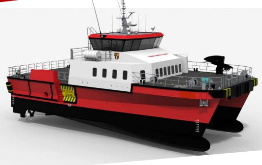
Designed by Walker Marine Design, UK — The MO9 was designed and built to perform a multitude of tasks, including crew transfer, offshore bunkering and cargo operations. Capable of transferring personal in 2m Hs, the MO8 is one of only a handful of vessels capable of achieving this milestone in passenger transfer.
