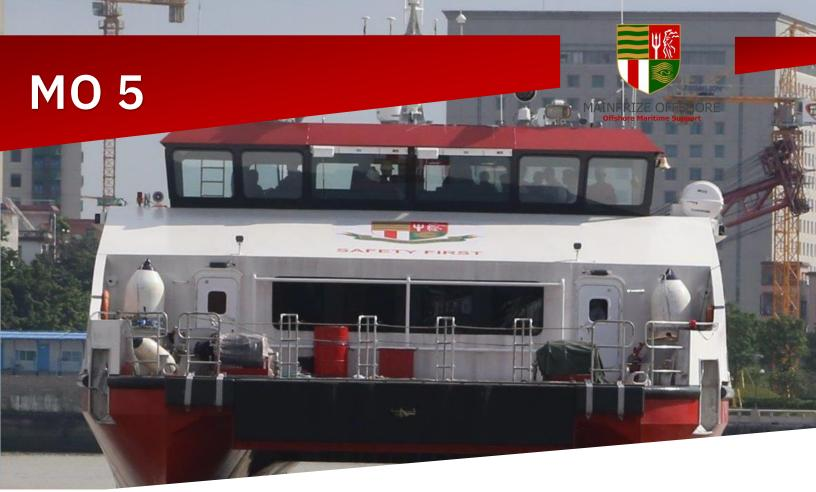
Designed by Walker Marine Design, UK — The MO5 was designed and built to perform a multitude of tasks, including crew transfer, offshore bunkering and cargo operations. Capable of transferring personnel in 2m Hs, the MO5 is one of only a handful of vessels that are capable of achieving this milestone in passenger transfer.
