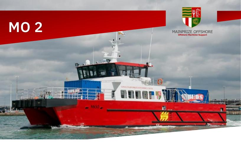
Designed by Tecknicraft, NZ – The MO2 was designed and built to perform a multitude of tasks, including crew transfer, offshore bunkering and cargo operations. Capable of transferring personnel in 1.75m Hs.
