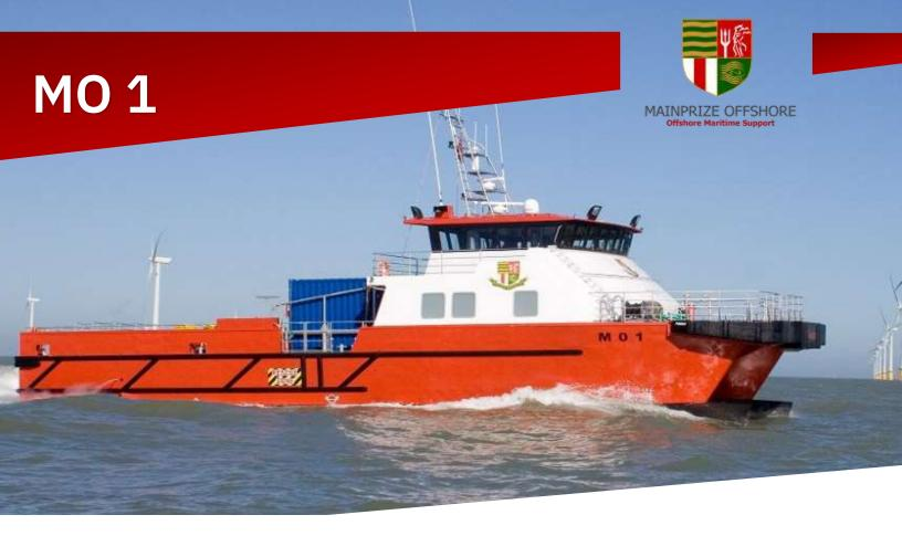
Designed by Tecknicraft, NZ – The MO1 was designed and built to perform a multitude of tasks, including crew transfer, offshore bunkering and cargo operations. Capable of transferring personnel in 1.75m Hs.
